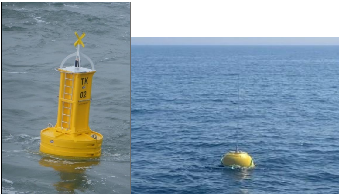
Figure 2: Navigation buoy and wave buoy.
